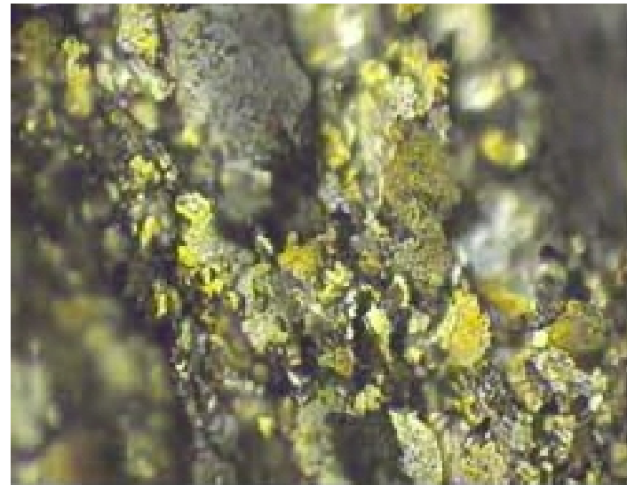
Figure 15: case hardened steel gear and bearing wear particles (120 \mu m max.) 200X
