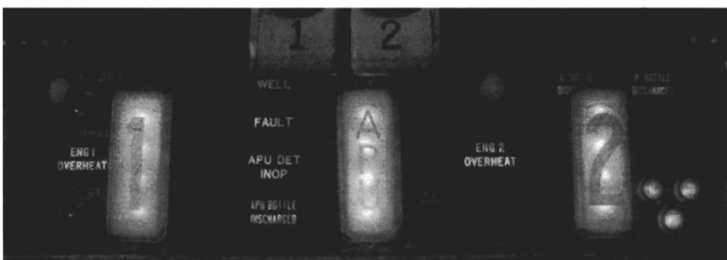
Figure 20.13: Typical fire extinguisher panel (B737)
