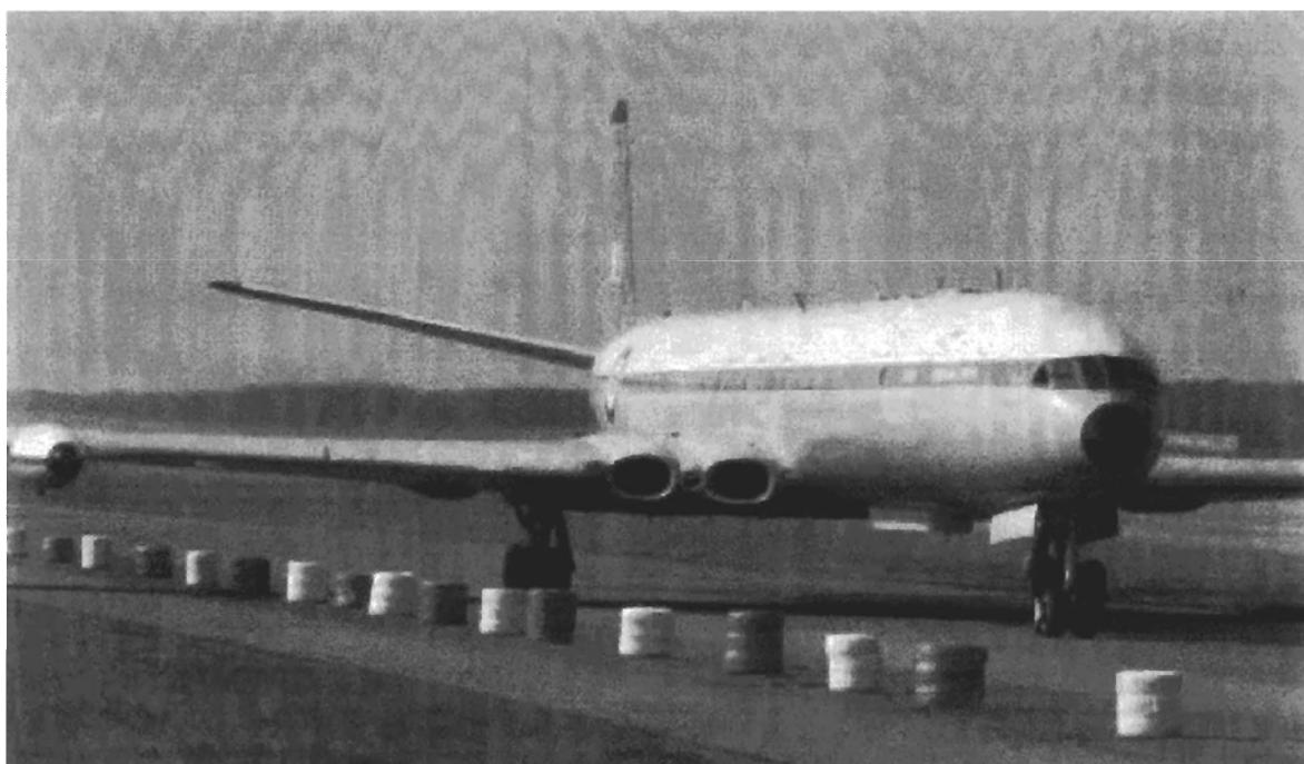
Figure 19.5: Integral wing root installation
