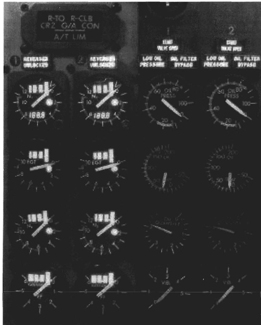
Figure 14.2: Analogue engine instruments (B737)
