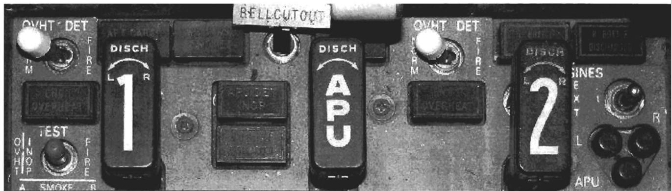
Figure 18.15: APU fire handle on main engine fire panel (B737)
