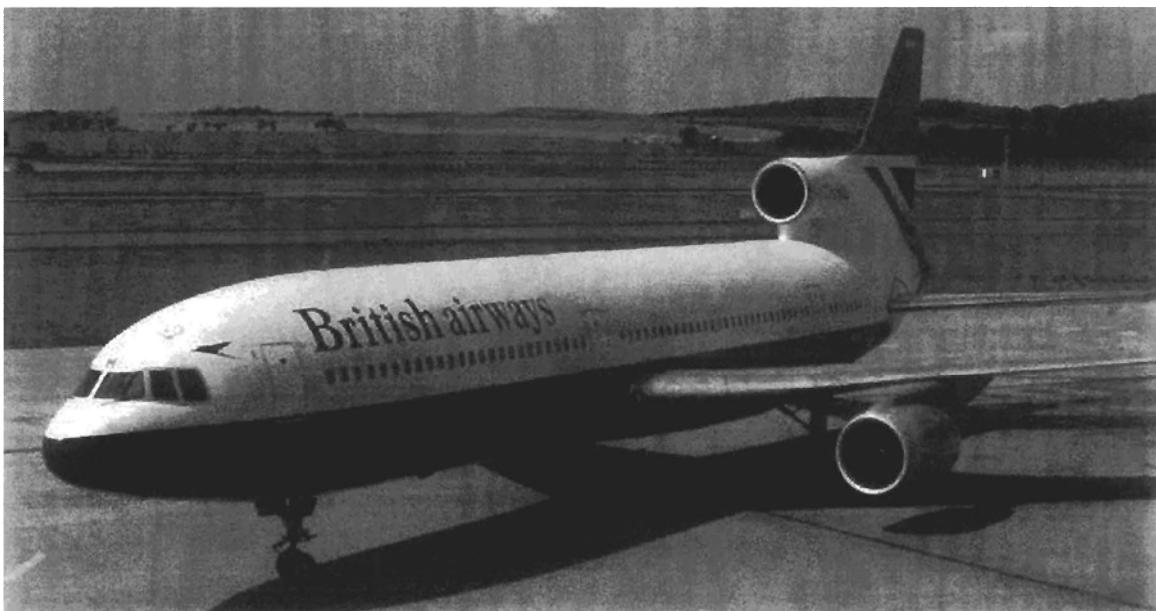
Figure 19.4: Tail and underwing powerplant installation
