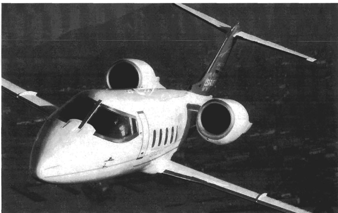
Figure 19.3: Tail powerplant installation
